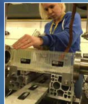
University of Manchester PhD student Agnese Lagzda setting up radiochromic films in a purpose-built water phantom to investigate dose penetration as the beam energy is varied.
